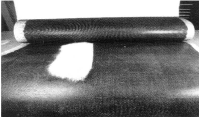
Figure 3. Extensive microbiological fouling of an RO element.
